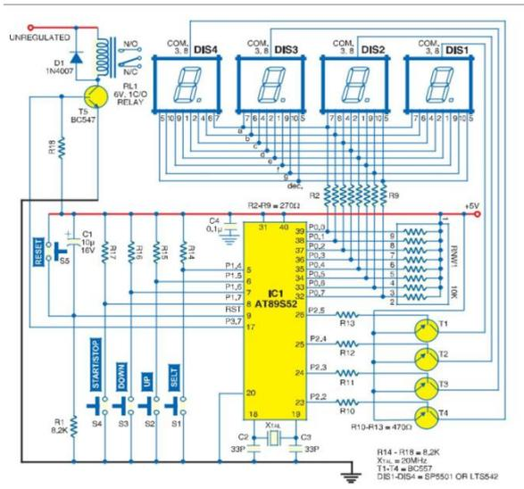
Figure 3: Circuit Diagram of Industrial Timer
